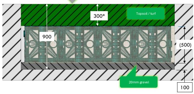
\* We recommend this depth as a minimum to maintain moisture levels directly above the void. However, to avoid differences in lawn colour, it is best to install in a none visual part of the garden, if possible.
