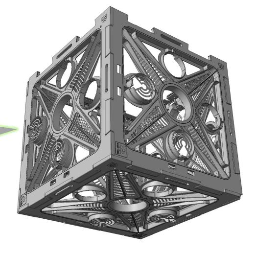
To install Internal Support Reverse 5-sided assembly as shown – open side up!
